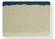
Microscopic cross section of an eGun™ sprayed WC-NiMoCrFeCo layer - Micro hardness 1228 HV0.3 - Porosity 0,2%
