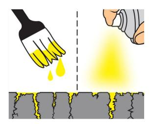
The FST TS-Sealer Products are materials designed to penetrate deep into the pores or cracks of thermal spray coatings. Once dried and cured, they form a protective barrier to gases and liquids that the coat is exposed to.
