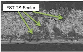
Sealers are recommended for porous coating systems, such as ceramics, that are designed to be used in liquid or atmospheric chemical environments, and for metallic coatings that have higher nobility than the substrate. Coatings that are anodic with respect to the substrate may be sealed to improve coating service life.
