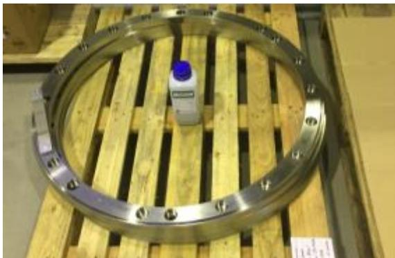
Not only did the coating quality improve, the total required spray time to finish the job reduced significantly. For example; for a 40" valve seat the coating time was reduced from approx. 1 hour to only 35 min. The reduction in coating time is the result of increased deposit efficiency, higher target efficiency and an increased spray rate compared to the JP5000.
