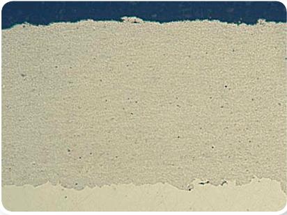
*Microscopic cross section of an eGun™ sprayed WC-NiMoCrFeCo layer
